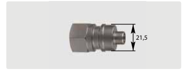
Plug : F. Hardened stainless steel. Max. 600 bar / 150 °C
