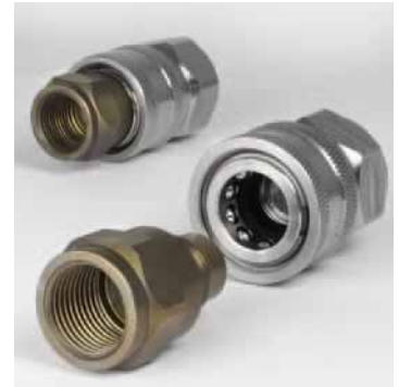
Plug : F. Hardened stainless steel. Max. 550 bar / 100 °C
