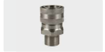
Coupling : M. Stainless steel. 60° cone. Max. 250 bar / 150 °C
