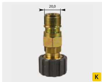
Plug : F. Zinc-plated steel + brass. Max. 250 bar / 150 °C
