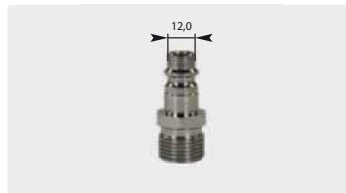
Plug : M. Ø 12 mm. Nickel-plated steel. Max. 200 bar / 100 °C
