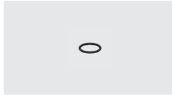
O-ring. (TYP) SP-20. 13.1x2.6. Max. 250 bar / 100 °C
