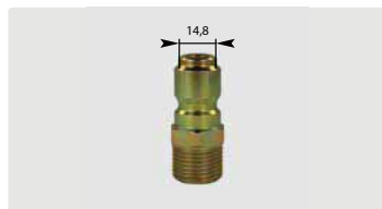
Plug : M. Ø 14.8 mm. Zinc-plated steel. Max. 150 bar / 100 °C
