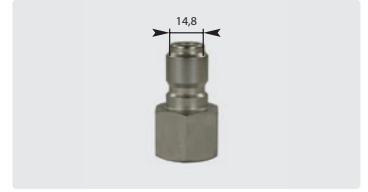
Plug : F. \varnothing 14.8 mm. Zinc-plated steel. Max. 250 bar / 100 °C
