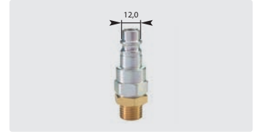
Plug : M. Ø 12 mm. Hardened steel, chemically nickel-plated / zinc-plated and brass. Max. 200 bar / 100 °C
