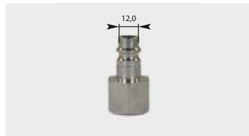
Plug : F. Ø 12 mm. Nickel-plated steel. Max. 200 bar / 100 °C
