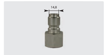
Plug : F. Ø 14.8 mm. Zinc-plated steel. Max. 250 bar / 100 °C
