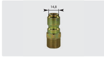
Plug : M. \varnothing 14.8 mm. Zinc-plated steel. Max. 250 bar / 100 °C
