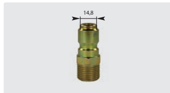
Plug : M. Ø 14.8 mm. Zinc-plated steel. Max. 250 bar / 100 °C
