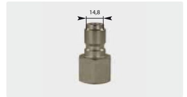
Plug : F. Ø 14.8 mm. Zinc-plated steel. Max. 150 bar / 100 °C
