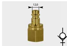
Plug : F. ∅ 12 mm. Brass. With valve. Max. 35 bar / 100 °C
