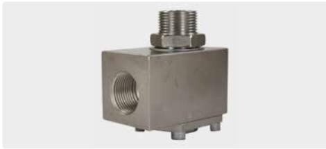
3/4" F : 3/4" M. DN 19. Housing and axle stainless steel. Max. 200 bar / 90 °C
