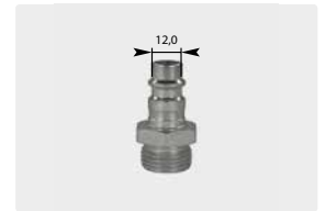
Plug : M. ∅ 12 mm. Nickel-plated steel. Max. 250 bar / 100 °C
