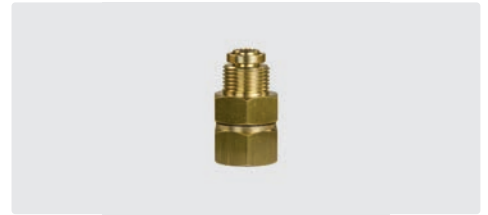
3/8" M : 3/8" F. Brass. Max. 220 bar / 90 °C
