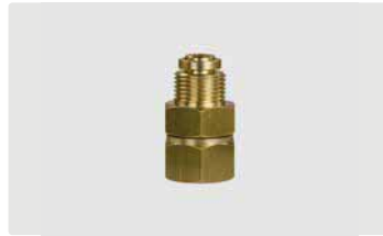
3/8" AG : 3/8" IG. Messing. Max. 220 bar / 90 °C
