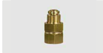
3/8" AG : 1/4" IG. Messing. Max. 220 bar / 90 °C
