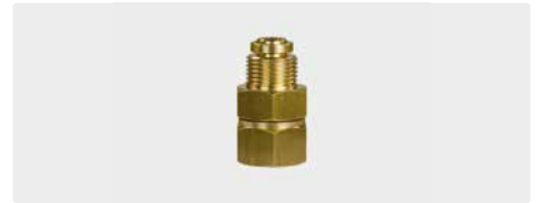
3/8" AG : 1/4" IG. Messing. Max. 220 bar / 90 °C
