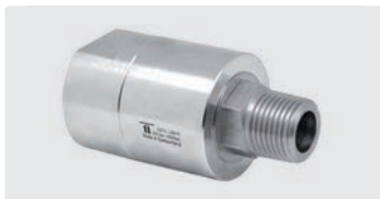
DGE. Housing nickel-plated brass. Single ball bearing system. Rust-proof. Max. 275 bar
